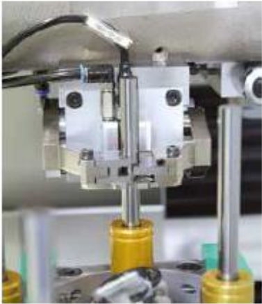
Blank being taken from chain loader.
