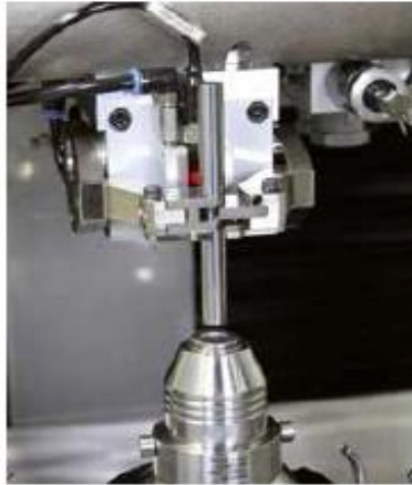
Pre-positioning for blank changing.
