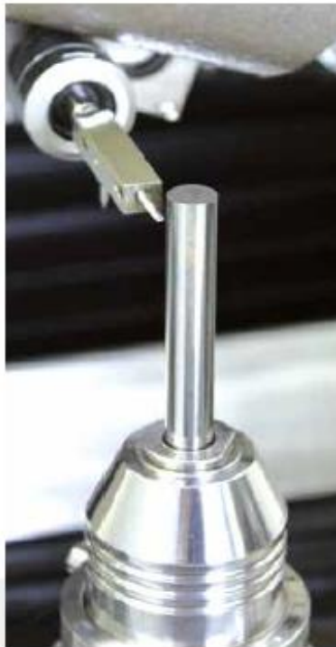
Pre-positioning for blank changing.
