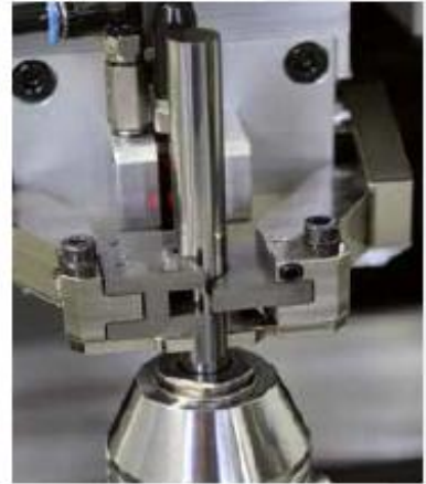
Reliable changing into hydraulic expansion chuck.
